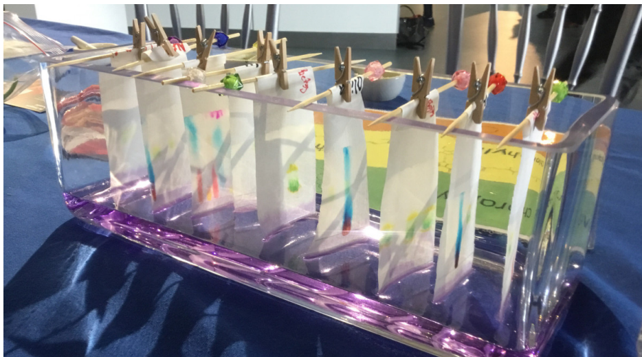
Chromatography. The pigments travel up the paper with the solvent front – the liquid acetone.
